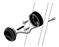
Figure 1. After installing the surface-mount plate, push the Kappa10.1t onto the mounting plate to snap it into place.
